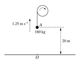
A load of mass 160 kg is pulled vertically upwards, from rest at a fixed point O on the ground, using a winding drum. The load passes through a point A, 20 m above O, with a speed of 1.25 m s<sup>-1</sup> (see diagram). Find, for the motion from O to A,
