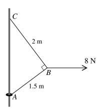
A small ring of mass  $0.2 \,\mathrm{kg}$  is threaded on a fixed vertical rod. The end A of a light inextensible string is attached to the ring. The other end C of the string is attached to a fixed point of the rod above A. A horizontal force of magnitude  $8 \,\mathrm{N}$  is applied to the point B of the string, where  $AB = 1.5 \,\mathrm{m}$  and  $BC = 2 \,\mathrm{m}$ . The system is in equilibrium with the string taut and AB at right angles to BC (see diagram).
